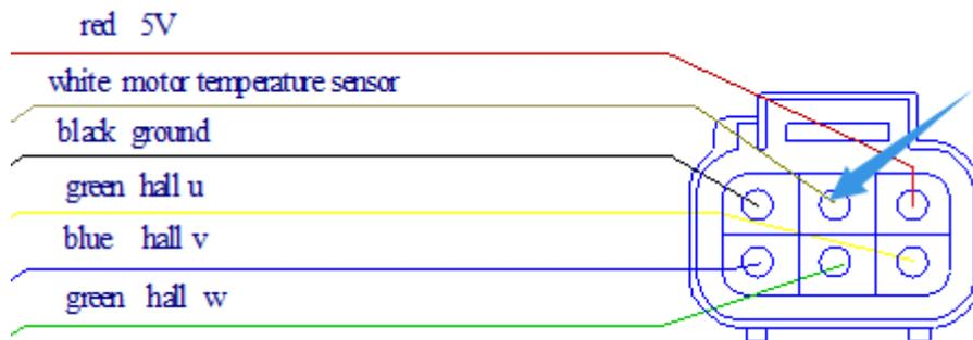
The controller support kty83-121 temperature sensor from motor inside. The function can be enabled or disabled from the software.
