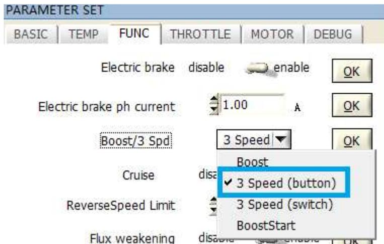
When select the 3 speed(button )in the software. use a button(which can be reset by itself) to connect the pink wire and ground wire.
