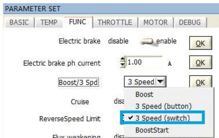
When select the 3 speed(switch)in the software. Use such switch to realize the 3 speed(switch) mode.
