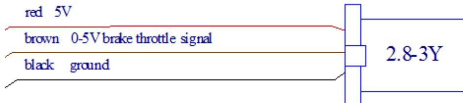
Use a separate throttle to connect to the terminal above. Please select the "Ebrake-throttle" mode, When spin the throttle ,the controller will enter the e-brake mode , the brake strength will follow the the throttle positon. the max streng can be set from "Electric brake phase current" as following:
